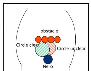
Thus Nero has the freedom to travel slightly to the left or right of the modified direction suggested by the LIDAR processor.
