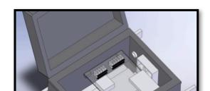
The primary design concern was to satisfy the following requirements: ensuring physical and electrical protection of the electronics and implementing a hardware-based wireless emergency-stop solution with an effective range of at least 50 feet that brings the robot to a quick and complete stop.
