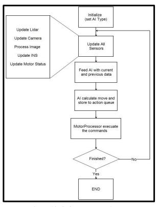
Figure 10: Software Flow Diagram
