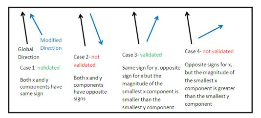
Figure 17: Validation of Modified Direction
